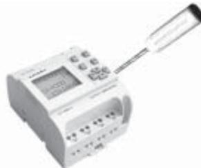
**Fig. 2.1 Remove LCD panel as instructed**
