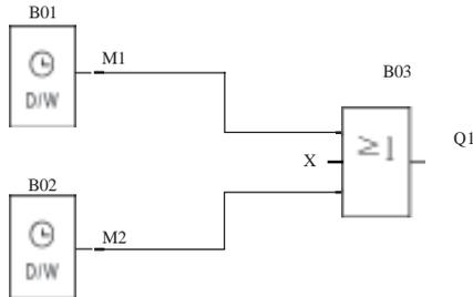
When FAB is used for the above control, it is very simple both in the connection of the external line and in editing the program. When QUICK II programming software is used for editing the control program, it is only necessary to set two time switch blocks.
