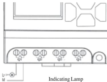
Fig. 2.1 Transistor Output
