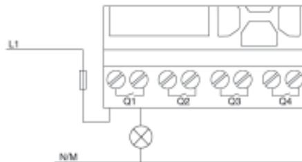
Fig 2.10 Relay Output
