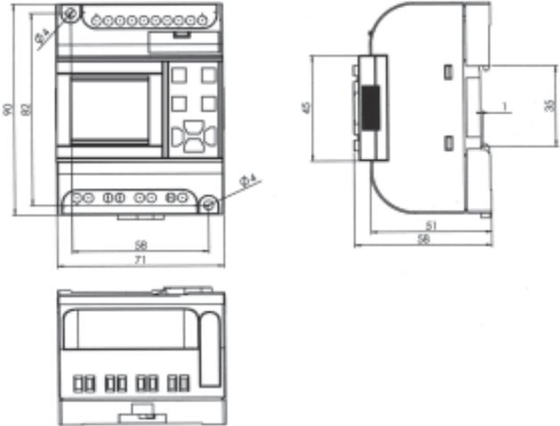
Fig 2.3 AF-10 FAB Series installation dimensions (Unit: mm)
