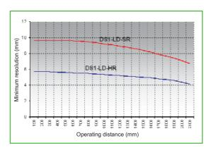
Variation of the minimum resolution according to the operating distance between the emitting and receiving units.
