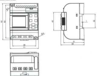
Fig 2.3 AF-10 FAB Series installation dimensions (Unit: mm)
