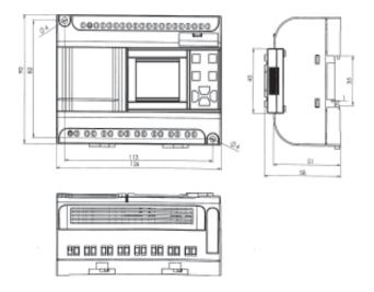
Fig 2.3 AF-20 FAB Series installation dimensions (Unit: mm)
