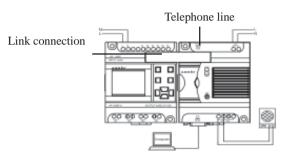
Fig 6.2 Connection Between FAB and AF-MUL
