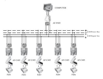
2) Assignment of FAB input/output points.
