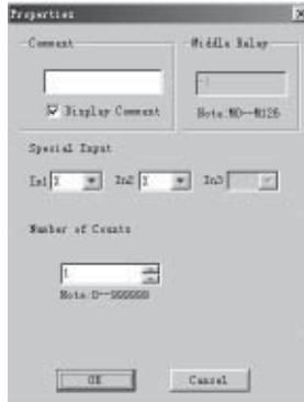
**Fig. 3.15 Setting Properties for Blocks with Counters**
