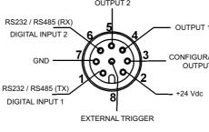
1 = white = RS232 / RS485 (TX) / Digital input 1 2 = brown = 24 Vdc 3 = Configurable output green = 4 = yellow = Output 1 5 = = Output 2 grey
